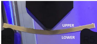
Fig 9. The upper part of the sample where the force-applied tip is, the lower part of the samples where the tip does not touch.
