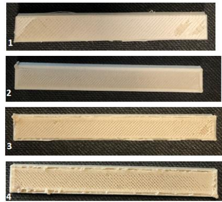
Fig 7. 3D printed flexural test samples numbered as 1. PC-10HA, 2. PC-15HA, 3. PC-20HA and 4. PC-25HA.
