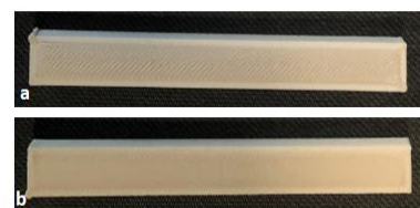
Fig 8. a) The top surface of PC-15HA sample, b) Bottom surface of PC-15HA sample which is contact with the heated table of 3D printer.
