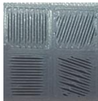
Fig 5. Default distances between the beads for different printing angles that are used in the paper.
