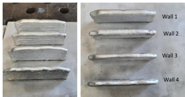
Fig 2. Four Walls produced by WAAM with different deposition parameters.
