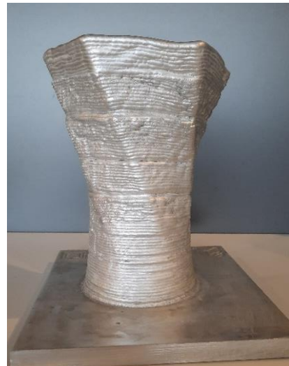
Fig 6. Deposited workpiece with changing cross-section from circle to hexagon.
