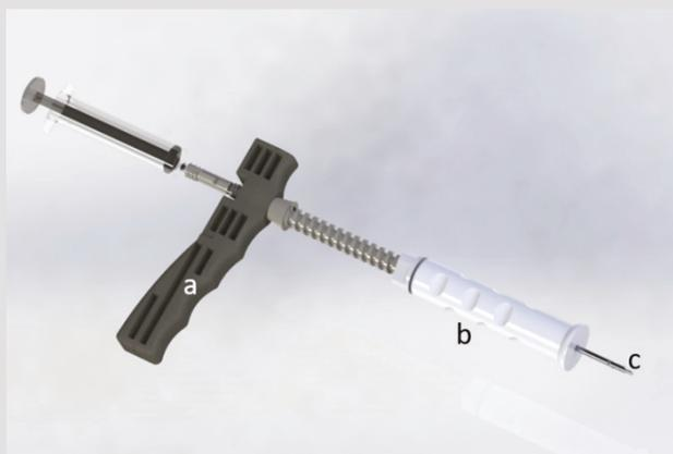
**Figure 2:** CAD model of the proposed injection device with ergonomic handle (a), depth limiter (b) and cannula (c).
