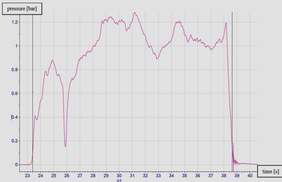
**Figure 3:** Pressure curve to determine the volume flow. Due the pressure changes cause by the manual injection an averaged pressure value has to be used.
