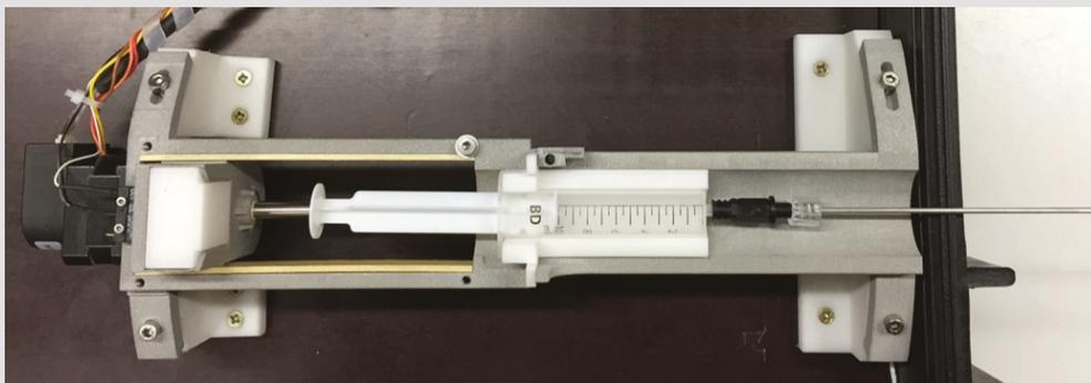
**Figure 5:** Construction of the test up to investigate the influence of the volume flow on the viability of the stem cells.
