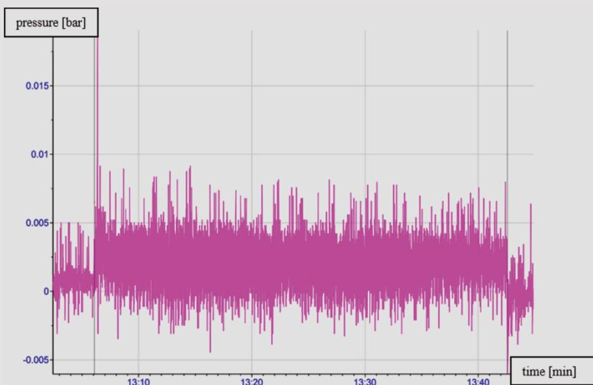
**Figure 4:** Pressure drop over the cannula. Due to the noisy measurement the use of an averaged pressured drop is necessary.
