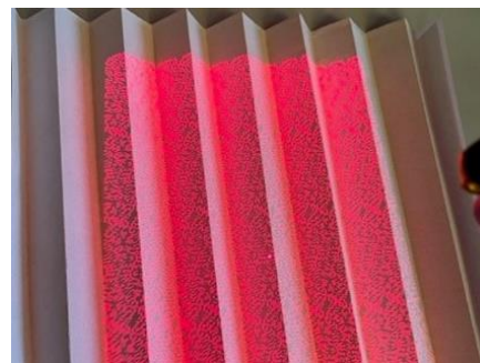
Figure 1: Photograph of a folded white paper and the laser projection (random pattern) as part of the experimental set-up A.
