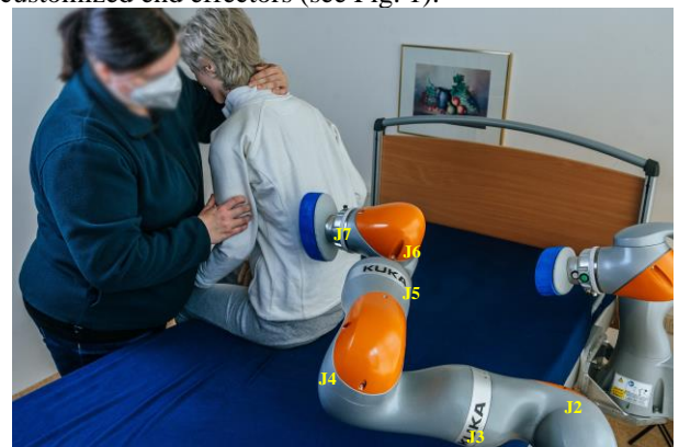
Figure 1: Patient simulator and robotic assistance system at the nursing bed with a padded end effector to support during patient repositioning processes. Individual robot joints are marked.
