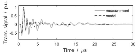
Figure 2: Transducer measurement compared to its simulation.
