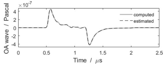
Figure 3: Computed OA wave compared to its estimation.
