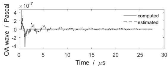
Figure 4: Computed and estimated OA using real measurements.
