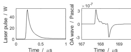
Figure 1: A laser pulse of 6μJ and the corresponding OA wave.
