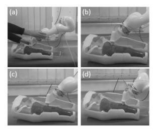
Figure 3: (a) The hand guidance mode allows to place the US probe on the leg phantom. (b)-(d) The robot arm moves along the leg, the artery center always in the horizontal center of the US image.
