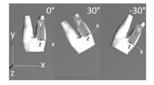
Figure 2: The world coordinate system (bottom left) and the end effector coordinate system after placing the US probe using the hand guidance mode for each rotation of the phantom. Note that the z-axes of both systems are always identical.
