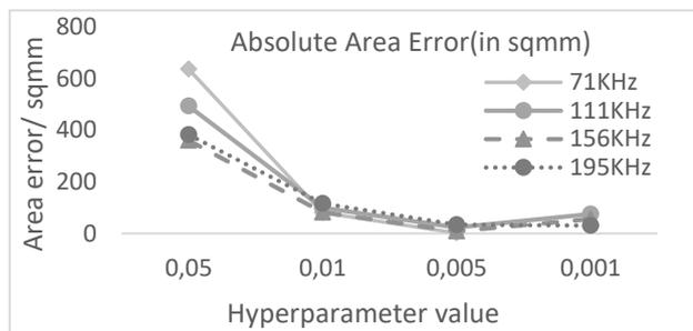
Figure 4: Area Error of tdEIT images when compared with actual cavity area for different hyperparameter values and frequencies.
