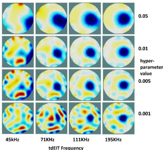
Figure 2: Reproduced EIT images for different hyperparameter values and frequencies.
