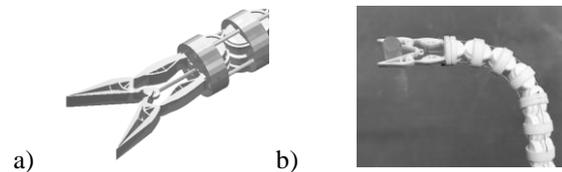
Figure 4: Realized compliant MIS forceps in a robotic system: a) 3D surface model of the realized forceps which is mounted to a tendon-driven soft robot structure, b) SLS-printed prototype of the forceps which is clamping an elastic tube.
