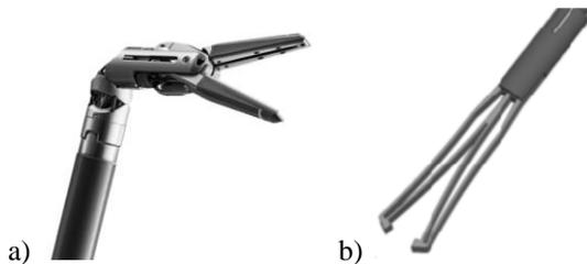
Figure 1: Rigid-joint-based and compliant MIS forceps: a) A rigid-joint-based forceps of the da Vinci surgical system [2], b) A compliant MIS forceps for robotic vitreoretinal surgery [3].
