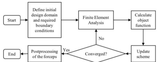
Figure 2: Workflow of the automatic synthesis method for MIS forceps, which is based on topology optimization.
