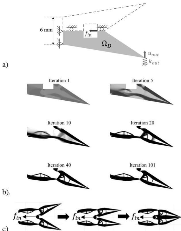
Figure 3: Automatic synthesis of a compliant forceps for robot-assisted MIS: a) Schematic representation of the design problem, b) Evolution process of the density during some iterations, c) FEM-simulation of the realized forceps under load  $f_{in}$  showing the deformation.
