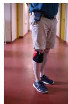
Figure 2: Setup with stimulator (on belt), cuff with stimulation electrodes, and one IMU on each instep (foot) below the laces (not visible).
