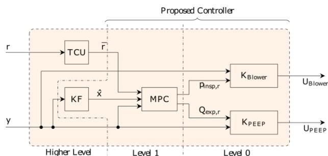
Figure 1: Proposed hierarchical control approach, with level 0 abstracting the nonlinear actuator dynamics and level 1 controlling the pressure level at the patient airway. Level 1 implements a linear robust model predictive controller (MPC) and a Kalman filter (KF). The higher control layer only contains the therapy control unit, which generates the reference.
