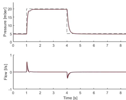
Figure 2: Expiratory pressure and patient flow of the simulated system with the nominal model parameters red and deviated parameters gray. The parameter were altered up to  $\pm 10\%$ , nonetheless the robust controller can track the dashed pressure reference.
