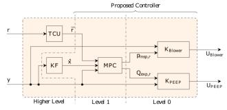
Figure 1: Proposed hierarchical control approach, with level 0 abstracting the nonlinear actuator dynamics and level 1 controlling the pressure level at the patient airway. Level 1 implements a linear robust model predictive controller (MPC) and a Kalman filter (KF). The higher control layer only contains the therapy control unit, which generates the reference.
