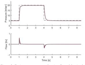
Figure 2: Expiratory pressure and patient flow of the simulated system with the nominal model parameters red and deviated parameters gray. The parameter were altered up to ±10%, nonetheless the robust controller can track the dashed pressure reference.
