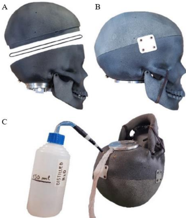
Figure 8: Third and fourth versions of the Instrumented Human Head Surrogate (IHHS 3.0 and IHHS 4.0) skull. (A) O'ring placement in skull surrogate, (B) final assembly of the skull surrogate components, and (C) distilled water insertion in the prototype.
