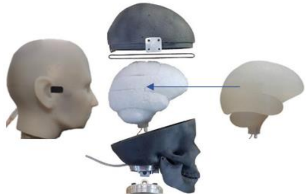
Figure 3: Skin, top skull, arachnoid trabeculae, bottom skull, jaw, and brain surrogates of the fourth version of Instrumented Human Head Surrogate (IHHS 4.0) developed by the DII (Dipartimento di Ingegneria Industriale) Department of the University of Padua.
