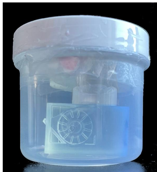
Figure 7: AP filled scala tympani of an aRWN with membrane inlay on top inside an airtight cup, filled with AP at its bottom and sealed with parafilm.
