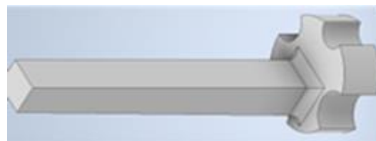
Figure 3: Positioner. The plunger like object holds the RNI in place above the RW opening between its round recesses and the inner membrane inlay wall.
