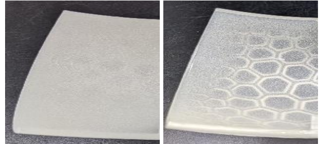
Figure 1b. Sharp edges and corners of unprocessed part (left) vs processed part (right)
