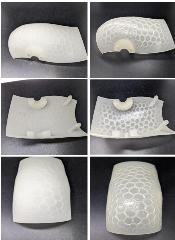
Figure 1a. Unprocessed part (left) vs Processed part (right). part used in this study are 20 cm in length, 9 cm in width, and 0.3 cm in thickness
