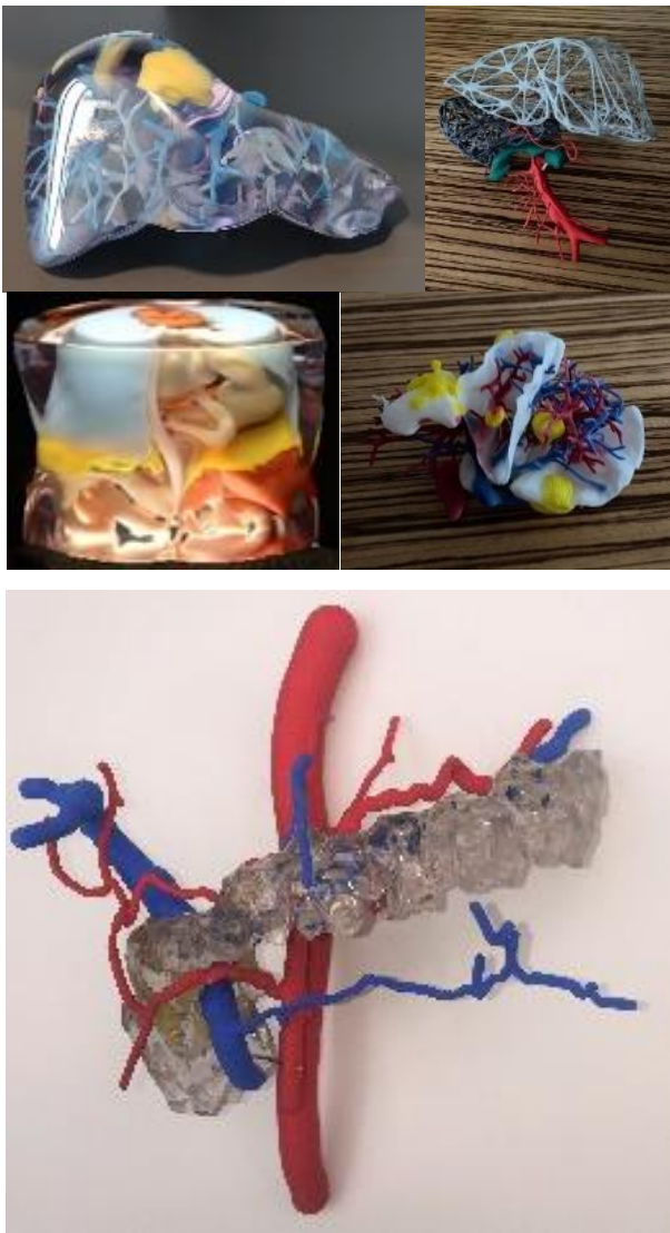
Figure 1: Different additively manufactured organ models: transparent liver, Polyjet® scale 50% (above left); liver and pancreas phantom, SLS, PA12 dyed in scale 100%(above right); Hernia phantom, Polyjet®, scale 30% (mid left); liver phantom, SLS, soft TPU dyed, scale 100% (mid right); Buehler Anastomosis, Hybrid SLS and Polyjet®, scale 100% (Below)
