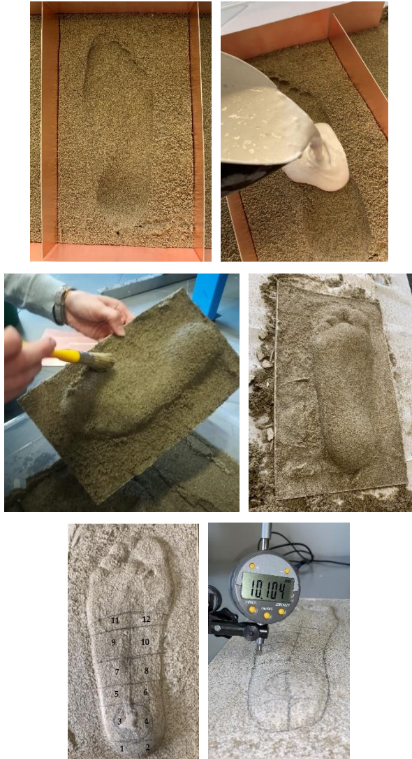
Figure 7: Sequence of the fabrication of the footprint mold, followed by the schematics of the foot region map and the mold characterization to measure the local height of the footprint.
