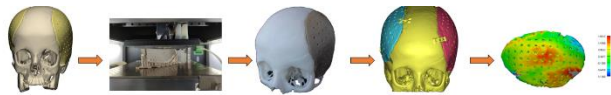
Figure 1: Schematic demonstration of the study evolution from left to right (1) implant design, (2) FLM additive manufacturing, (3) assessment of the implant with anatomical model (4) assessment of the implant radiography after implementation (5) dimensional comparison
