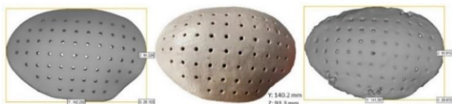
Figure 2: Dimensional validation from left to right (1) implant design footprint, (2) FLM additive manufacturing dimensional analysis (after post-process), (3) dimensional analysis of the implant segmented from the CT image taken after implantation
