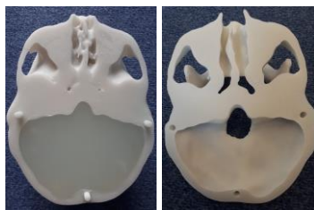
Figure 2: Left, a photograph of the 3D printed upper part of the phantom. Right, a photograph of the 3D printed lower part of the phantom.
