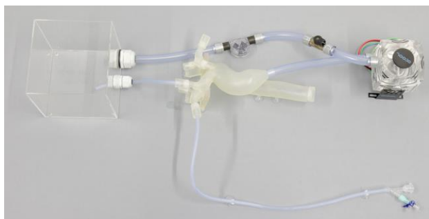
Figure 1: Overview of the simulator. With water reservoir, 3d printed aortic arch and pump (from left to right).
