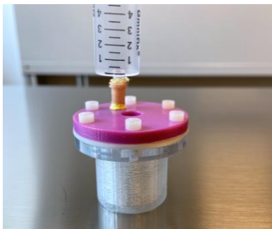
Figure 3: Fully assembled actuator with a 10 ml syringe connected to the pneumatic actuator via Luer lock adapter. Vessel phantoms can be threaded through the hole in the magenta lid.
