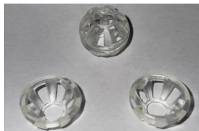
Figure 4: 3D-printed tissue holder fabricated with Form 3B and resin Surgical Guide VI.
