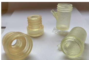
Figure 3: 3D-printed rinsing chamber fabricated with Form 3B and resin Surgical Guide VI.
