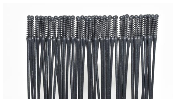
Figure 1: Nasopharyngeal Swabs produced via MJF powder-based method and vapor smoothed with PostPro3D
