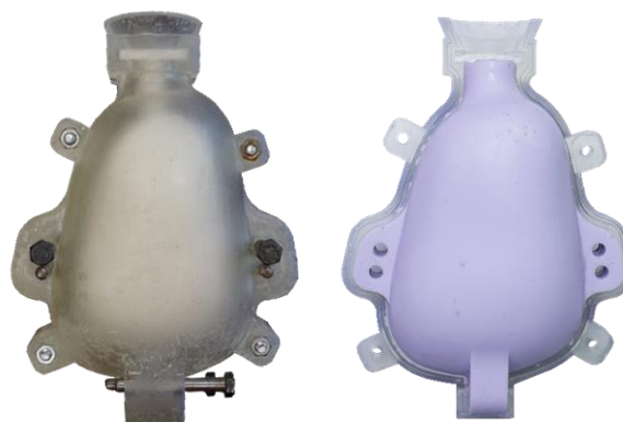
Figure 3: Assembled bladder mold (left) and silicon model of bladder wall (right).
