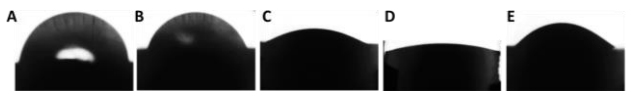
Figure 3: Contact angle of [A] PLA and [B-E] PLA scaffolds incubated with PDA for 10 min, 30 min, 2 h and 24 h respectively.
