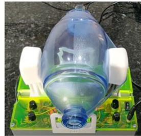
Figure 3: Resultant operational automated ventilator device.
