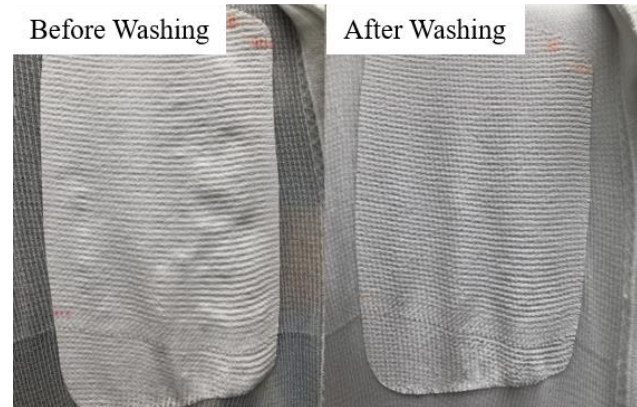
Figure 3: Image of single layer of polyurethane interfacial layer before and after washing cycle.
