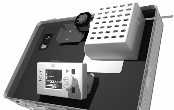
Figure 1: View of the FilVer . The control unit is visible in the front. At the back behind it is the extrusion path with the integrated force measuring unit.
