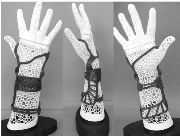
Figure 3: Wrist orthoses generated by benchtop SLS-printer LISA a) direction of view on the back of the hand, b) lateral view of the thumb, c) view of the palm of the hand
