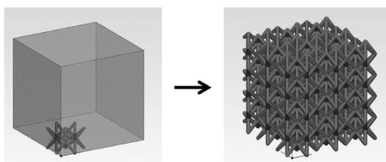
Figure 2: star like structure in the cubic body
