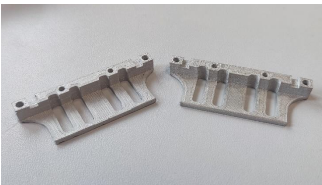
Figure 5: Metal MEX manufactured sensor parts after the sintering process
