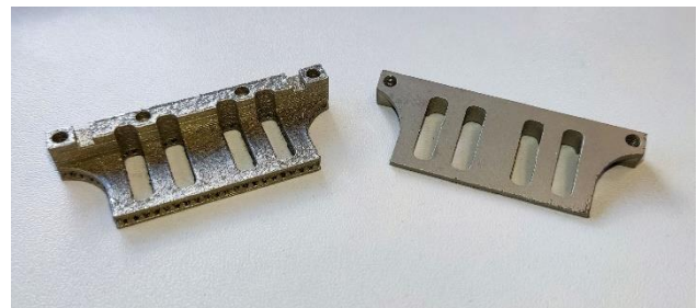
Figure 6: LPBF printed sensor parts as-built (left) and after glass bead blasting (right)
