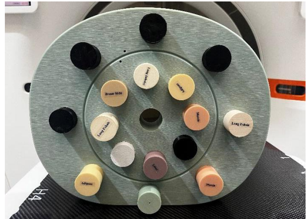
Figure 3: Set-up of the AM truncated cones placed inside the calibration phantom together with the changeable material inserts.
