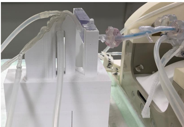
Figure 3: Integration of the MMA model with holder into the existing vessel tree of the simulator HANNES
