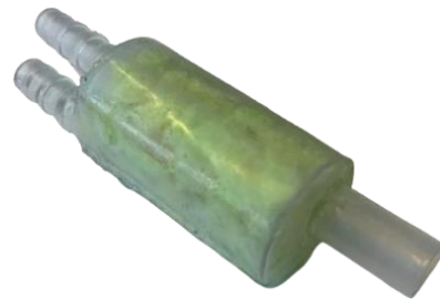
Figure 3: Manufactured rupture model, consisting of an additively manufactured housing and a subarachnoid space filled with sponge.
