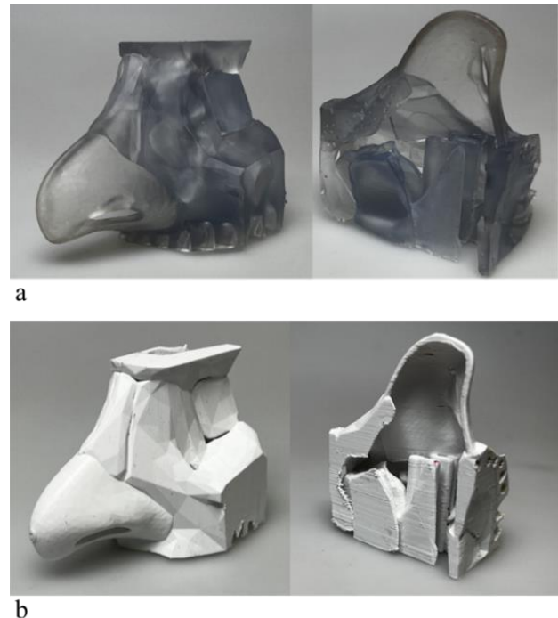
Figure 2: 3D printed anatomical test models for the second test phase. a See-through Flexible 80A. b White PLA.
