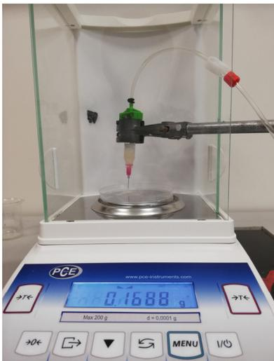
Figure 3: Test Stand for flow rate measurements of the silicon rubber.
