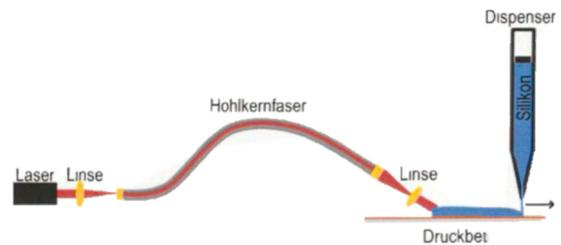
Figure 1: principle of printing silicone rubber with ultra-fast laser curing [3]
