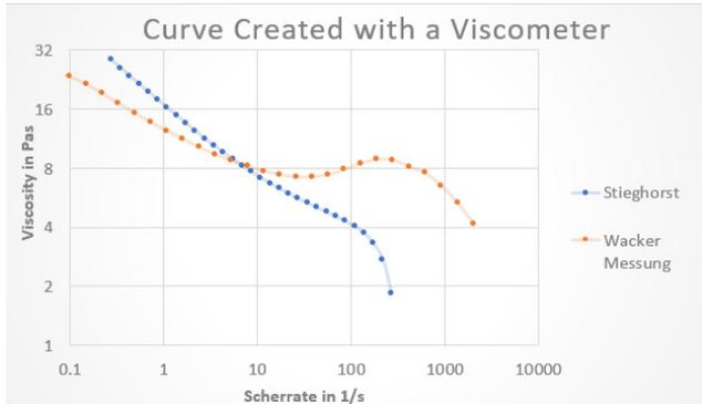
Figure 2: Viscosity measurements in relation with the shear rate of the silicon rubber
