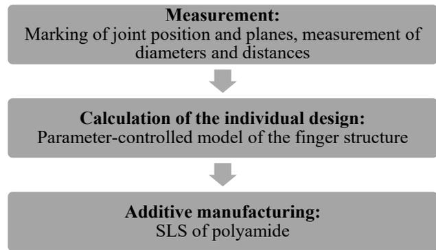
Figure 3: Process of making individual hand exoskeletons: First the hand's anatomy is measured, then the individual design is realized by a parameter-controlled model of the finger structure and finally, the exoskeleton is manufactured by SLS of polyamide.
