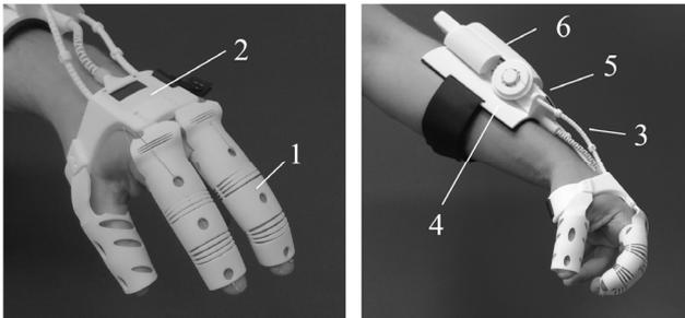
Figure 2: Prototype of the hand rehabilitation device: Finger overtube (1), finger base unit with display (2), Bowden wire (3), pulley (4), buttons (5) and actuation unit (6).
