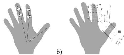
Figure 1: (a) Kinematic model of the hand exoskeleton (distal and proximal interphalangeal joints). (b) Position of measurements defined by planes perpendicular to the finger axis.
