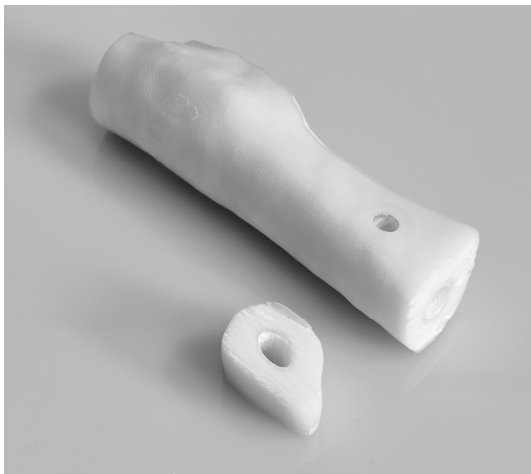
Figure 3: Anatomic bone model 3D-printed from VisiJet M3 X
