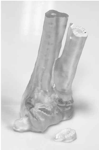
Figure 2: Anatomic bone model printed from Clear Resin
